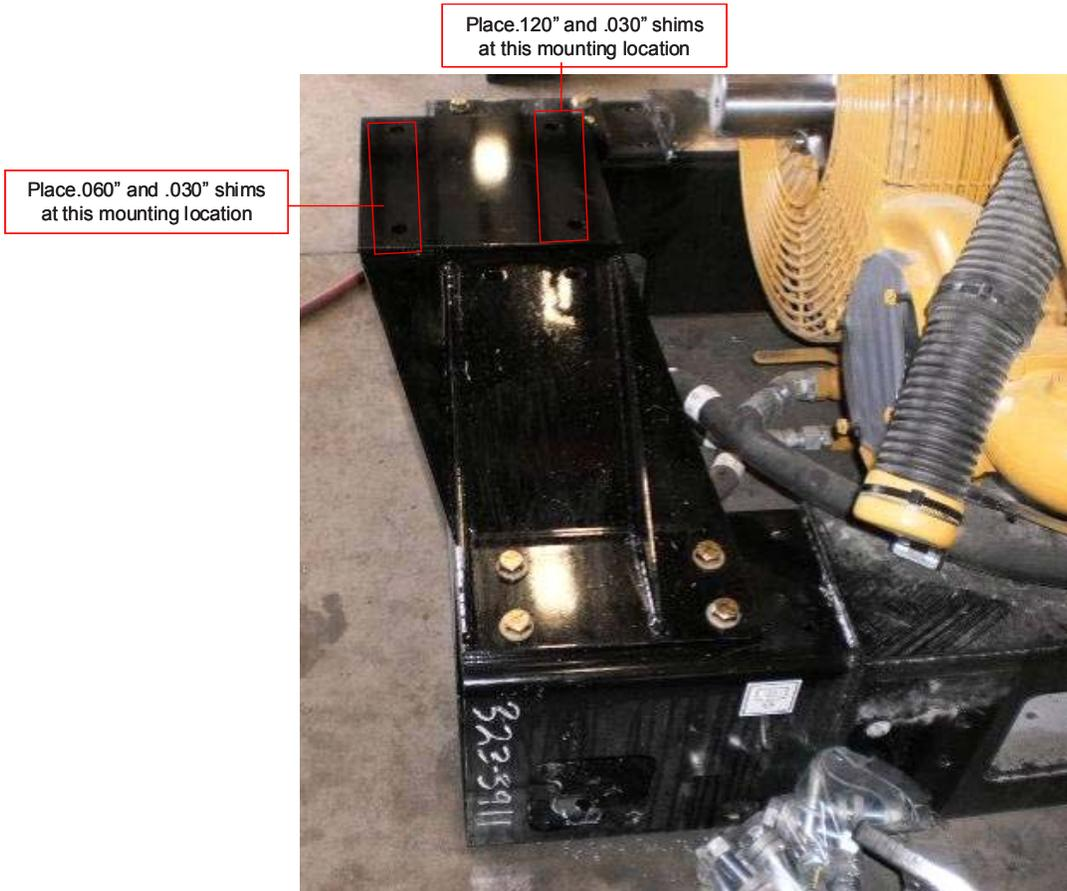
**Figure 7: Bearing shim selection and locations**
