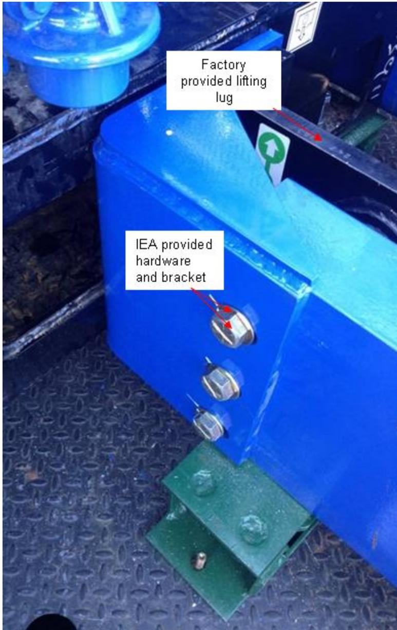
Figure 12: Engine rail to wishbone interface (outside view)
