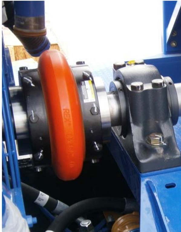
**Figure 14: Flexible coupling installed**
